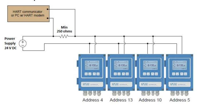
A single minimum 250  $\Omega$  resistor (maximum 800  $\Omega$ ) is needed to communicate with all the instruments connected to the bus, and each of them must provide 4mA.
