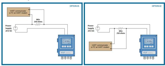
An external minimum 250  $\Omega$  (maximum 800  $\Omega$ ) resistor is needed in order to communicate with HART protocol.
