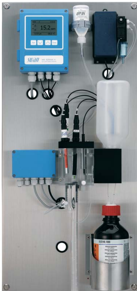
Figure 2b: Sodium analyzer with active reagent addition for sodium measurement in low pH samples.
